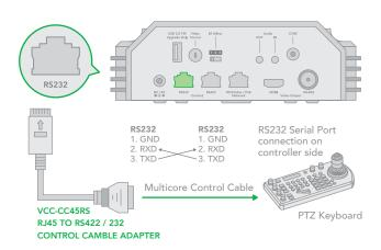
11. Or you can use CAT5/6 network cable (T-568B standard pinout) to make RS232 connection by following the pin definition below:
