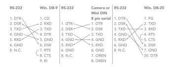
Use extension cables included RJ45 to RS232 8 pin Mini Din adaptor to make RS232 connection for your control device.
