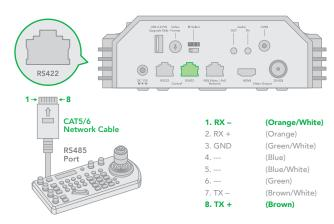
How to make RS485 multiple cameras connection with RS485 standard serial port controller:
